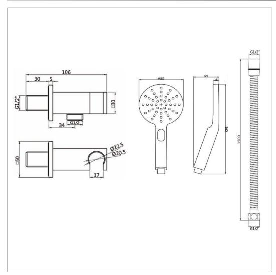
Fuse Wall Outlet and Handset Holder Kit
